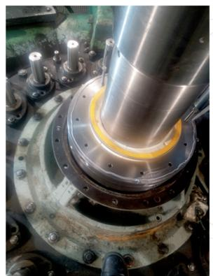
In a first for its Latin American operations, Thordon Bearings has supplied a water-lubricated SXL turbine guide bearing and segmented shaft seal to state-owned power company Empresa Provincial De Energía de Córdoba (EPEC) in Argentina.
