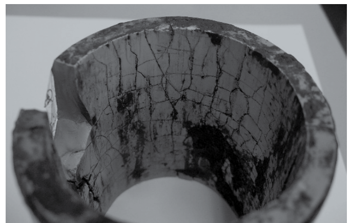
Typical example of ThorPlas bearing with hydrolysis.
