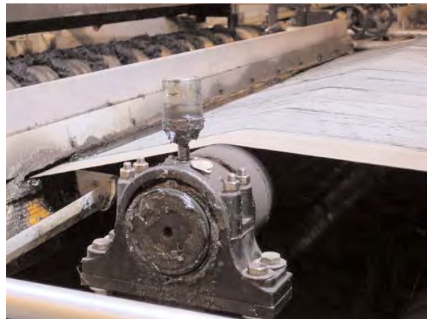
Pillow block bearing on filter press
