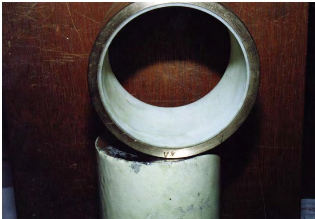
Test bearing and spool after 38,000 test cycles
