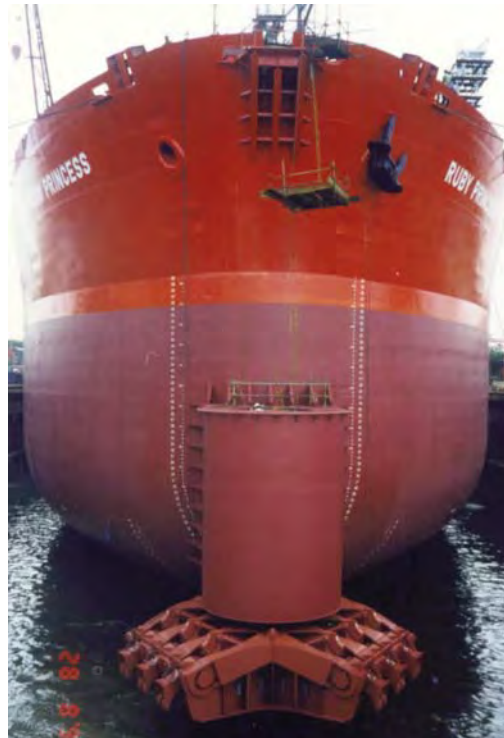
Bow turret installed on Ruby Princess with SXL turret mooring bearing
