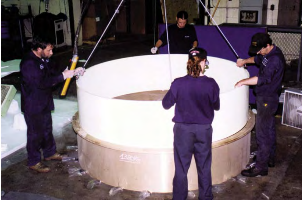
Installing SXL into bronze carrier
