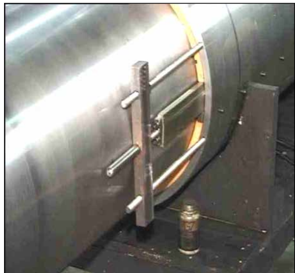
Figure 4. Single Key removal using key extraction tool
