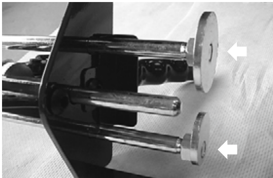
Figure 4: Plungers in manual gun (see arrows)
