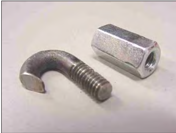
Figure 5. J-hook and nut used to remove bearing segments (yard supply)
