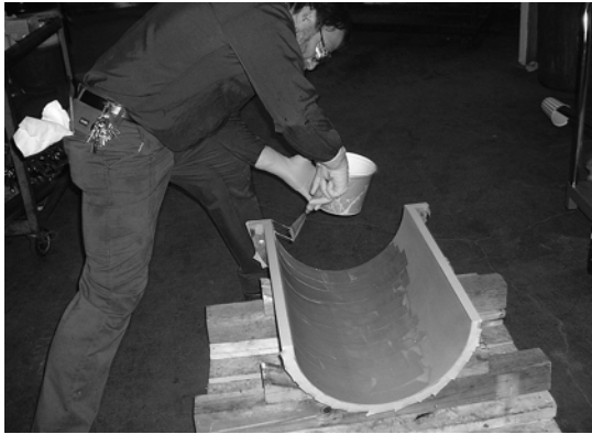
Figure 5: Adhesive applied to split metal housing.
