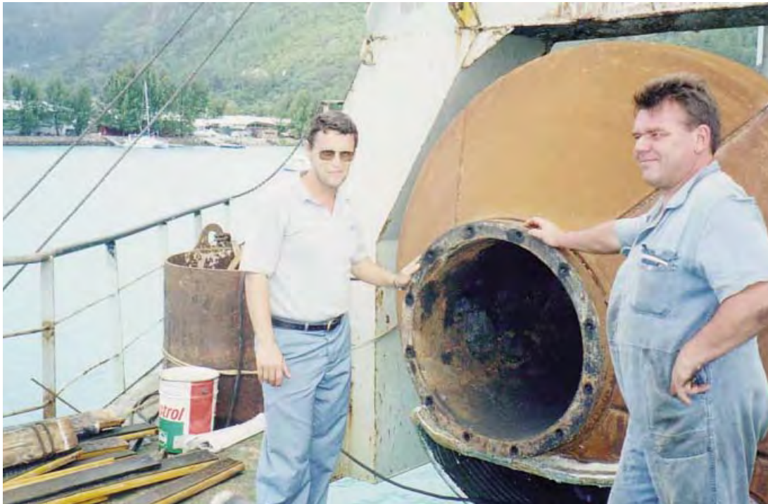
Cutterhead Housing of Dredger M/v Vesalius, housing diameter 730.25mm
