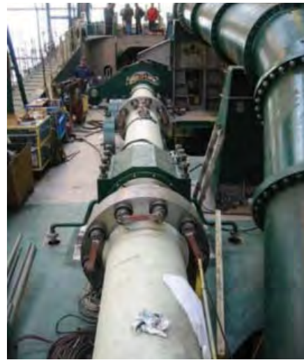
Cutterhead shaft line showing 2 of 3 Composite intermediate bearings
