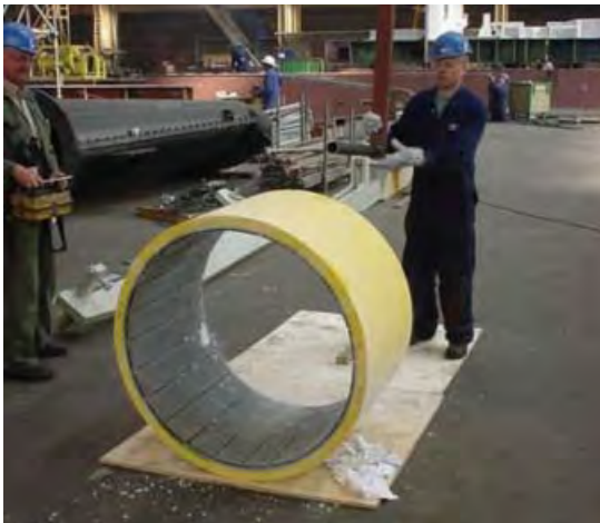
Composite cutterhead shaft bearing removed from dry ice and ready to be installed in housing
