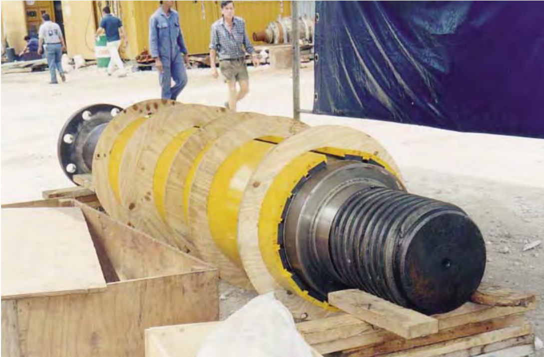
Thordon Composite staves installed in test housing (except the 18th long and short stave) on a spare shaft prior to installation
