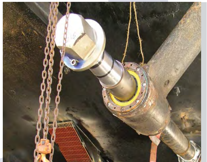
At current wear rates, Thordon RiverTough bearings are expected to last over 10 years
