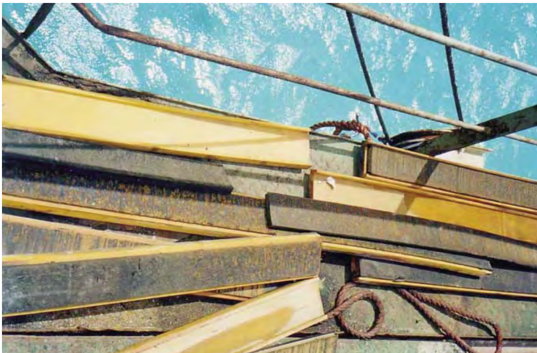
Thordon Composite staves originally installed in February 1996 were removed after over five years of operation
